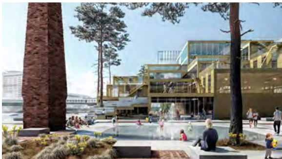
Figure 34: Waterside, Belfast – use of computer-aided design of built form to create public spaces that mitigate wind and rain to extend the usable outdoor season (Henning Larsen)
